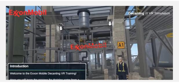
Decanting is a critical process in which water needs to be carefully separated and drained from a liquid propylene tank. Failure to do this properly can critically injure personnel, as well as leaking propylene into the sewage and filtration systems. View video: <u>https://youtu.be/YBy3TV\_liag</u>
